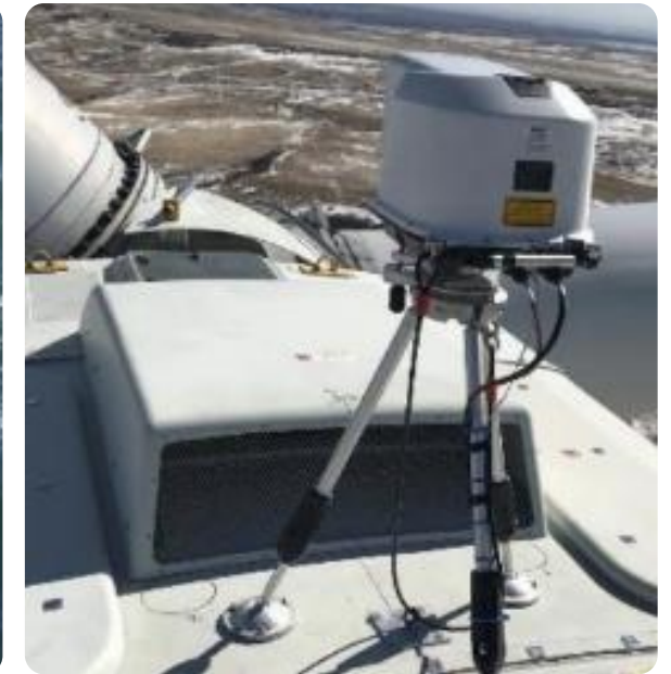
Nacelle-mounted Scanning LiDAR
